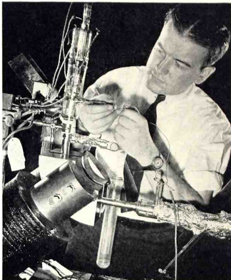
The key part of the instrument—a curved glass tube fixed between the poles of an electromagnet. The magnet draws electrified molecules traveling down the tube so that only those having a certain mass, or weight, go around the curve and hit the target. At the target they are collected and their electrical charges counted by meters, enabling an accurate check of the composition of the mixture.
