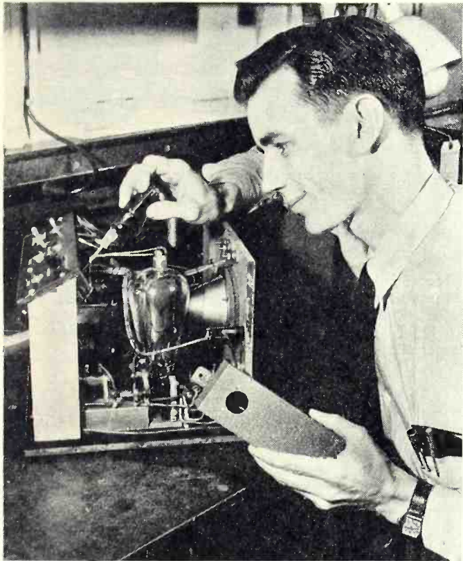
G.E. engineer shows the inside of the portable millionth-of-a-second flashlight unit for use in photography.
