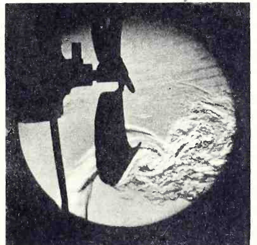
A one-millionth of a second exposure, of a stream of heated air being drawn through a fan revolving at 1800 r.p.m.
